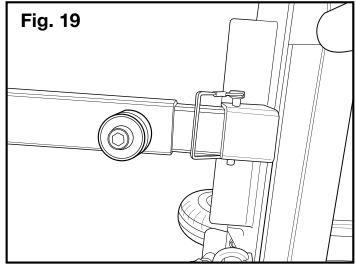
10. Place the roller guides at 4 to 5 foot spacing or two guides per section. Adjust spacing as required. The size/number of wires, degree of change in direction and elevation will dictate placement and the actual number of guides needed. Once located, swing bottom metal tab 180 degrees out from its locked position and place on tubing (Fig. 20). Once roller is placed on the tube swing bottom lock tab back 180 degrees and tighten by turning locking knob clockwise to secure in place (Fig. 21).
