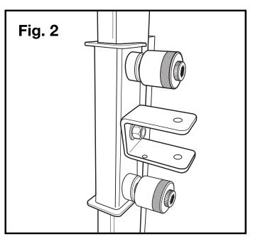
2B. Working your way back from the conduit, select a piece of tubing (Fig. 3) and insert end into the "C" Clamp and turn locking knob clockwise until tight (Fig 4A). For Panel Can Adaptor, align holes in tubing with bracket on adaptor and install supplied pin (Fig. 4B)
