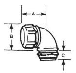
Ideal for cramped locations or tight corners where large radius conduit elbows will not fit or would appear unworkmanlike. Shoulders on body of 1/2" size are hex-shaped to provide positive holding for standard installation tools. Use insulated type for simple, and safe, installations. Malleable iron. CSA rated 105°C.
