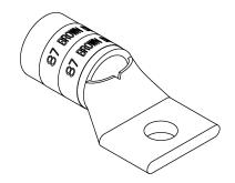
WIRE SIZE: 350 WELD, 400 WELD, 500 MCM MATERIAL: HIGH CONDUCTIVITY COPPER FINISH: TIN PLATED
