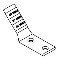
WIRE SIZE: 350 WELD, 400 WELD, 500 MCM MATERIAL: HIGH CONDUCTIVITY COPPER
