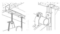
Pipe section hangs from D-990 concrete insert.
