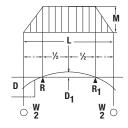
Beam continuous over two supports Two exterior symmetrical loads
