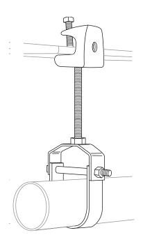
500 Series Beam Clamp supports pipe with C-710 clevis hanger.
