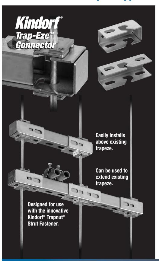
The innovative Kindorf® Trap-Eze™ Connector changes a time-consuming retro-fit trapeze application into a streamlined process. Using a Kindorf® Trapnut® Strut Fastener, the new Trap-Eze™ Connector can be easily installed above or to the side of an existing assembly, eliminating the need to disassemble and reassemble the trapeze. It is designed for use with shorter strut lengths that can vary in length by as much as an inch, so the strut can be rough cut versus laborintense precision cut.
