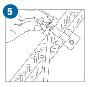
Apply locking device and tighten screw moderately.
