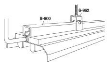
Channel raceway system supports and feeds fluorescent lighting fixtures.
