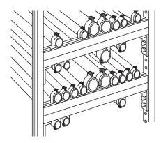
Steel beam mounting application. Aluminum straps with stainless steel hardware. Frame assembly carries multiple conduit runs.
