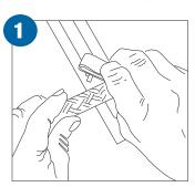
Insert pin of strap in slot of hanger.
