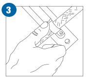
Push strap and cable to end of hanger slot so tongue of strap hooks below slot.
