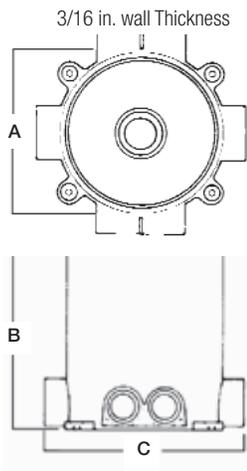
The 68-P floor box provides flush service for power, communications and data. The nonmetallic floor box is used in concrete floors and is suitable for **carpet, tile or wood applications**.
