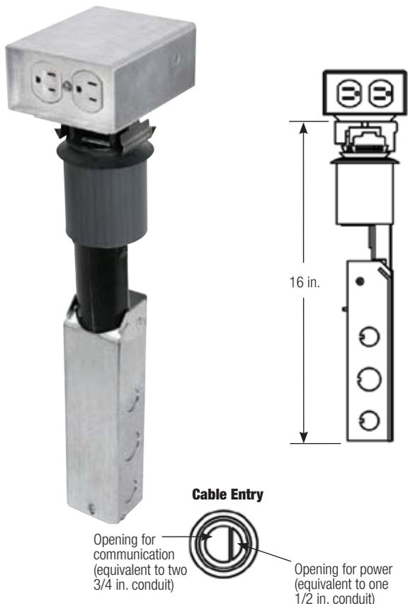
By mounting all outlets above-floor level and at a 90° angle to the floor, the FPT Pedestal Series protects power receptacles and communications devices from dirt and debris. An overhanging housing provides additional protection for the outlets.
