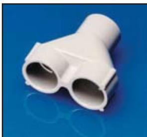
The 3/4 in. Y Fitting provides for in and out service from a single 1 in. port and allows for two 3/4 in. parallel conduit runs to adapt into a single conduit body port.
