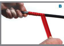
Wrap along the centerline with as much tension as possible. When the tape touches the previous layer, it will stick and hold.
