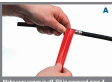
Make sure power is off. Fill in recessed gaps if needed. Cut an easy to handle length of tape and stretch the tape half its width from the start.
