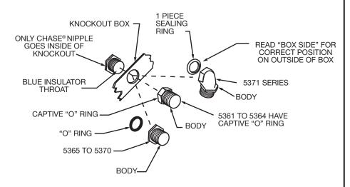
Lock-up Can Be Made By Tightening Chase® Nipple To Body Or By Turning Body Onto Chase® Nipple
