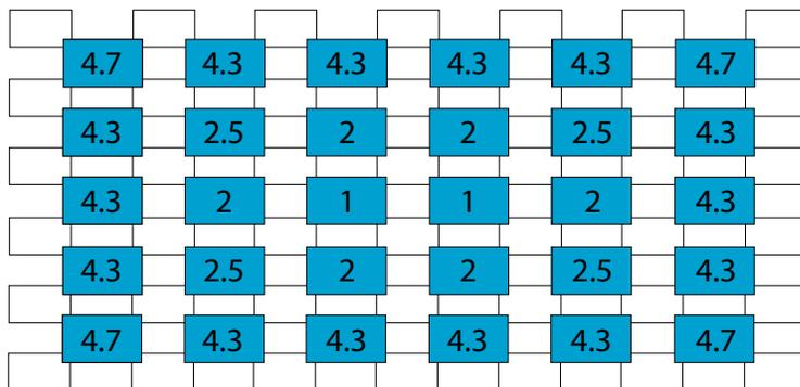
For a bay on the very perimeter edge of the array that supports 2 panels only contributes half of its weight to each panel it supports. The same goes for an interior bay that supports 4 panels, it only contributes 1/4 of its weight to each panel. After rounding up to whole blocks the resulting final ballast distribution is as follows:
