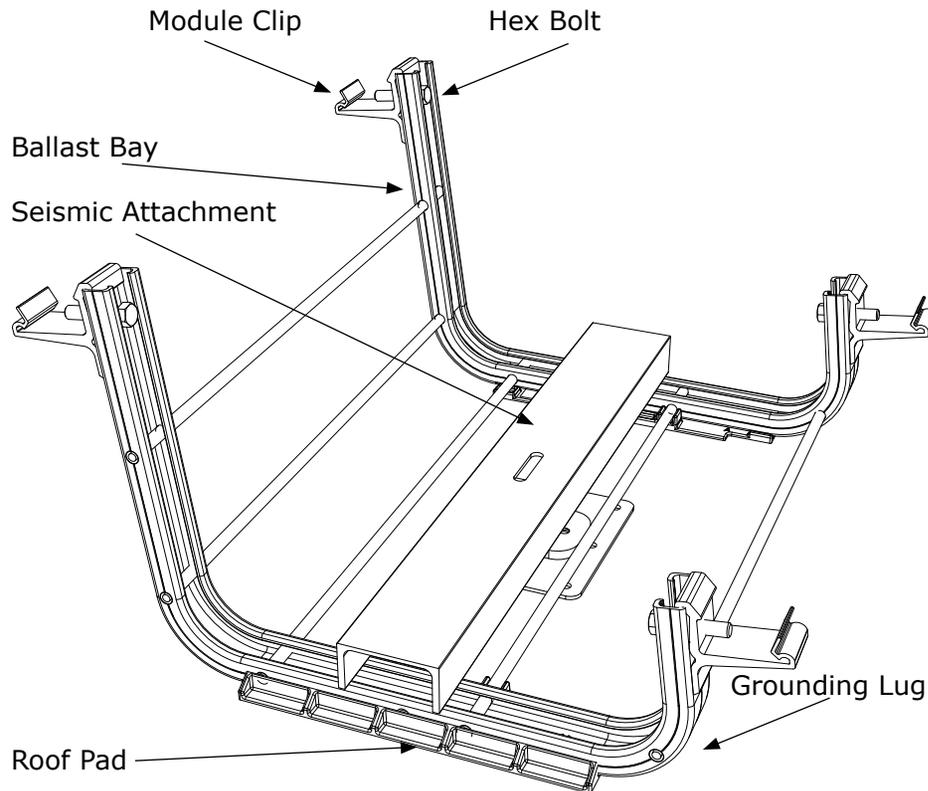
**Ballast Bay:** Supports the PV module and holds the ballast blocks. The Ballast Bay supports four interior modules, two edge modules and one corner module. It contains a maximum of 3 full size ballast blocks (4"x8"x16").
