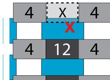
In this case you need 3 total bays in the area where the "12" is. In this case you put 2 bays with 4 blocks a piece in the "12" area and then add an additional bay with 4 blocks where the red "x" is.
