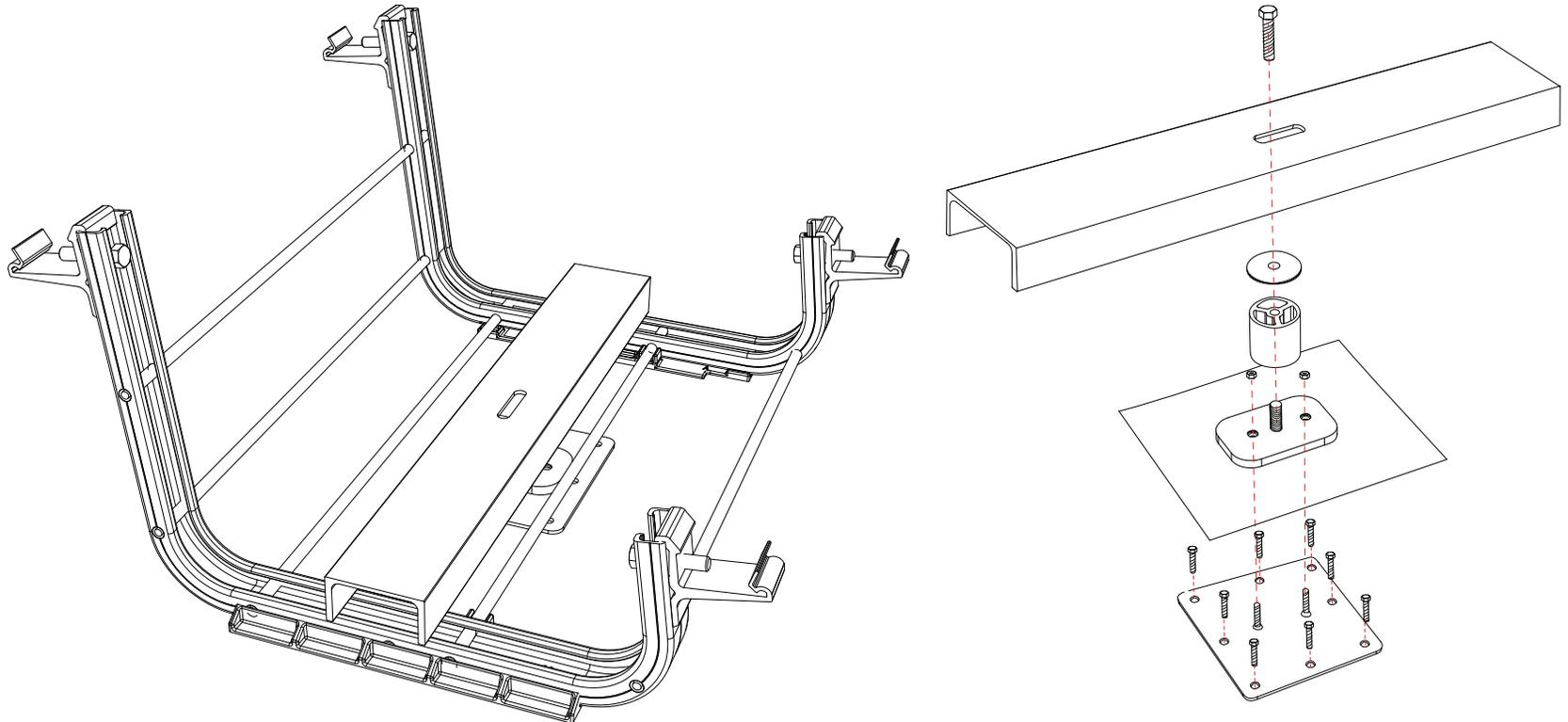
Material (clamp bar & standoff): 6105-T52, 6063-T5 Aluminum extrusion
