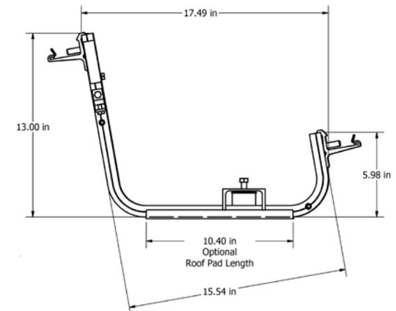
Material: 6105-T52, 6063-T5 Aluminum extrusion
