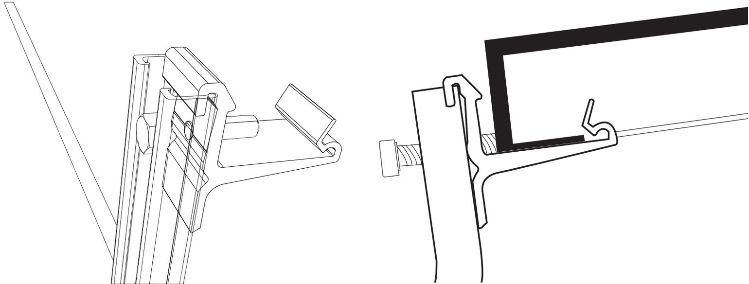
Material: 6105-T52, 6063-T5 Aluminum extrusion
