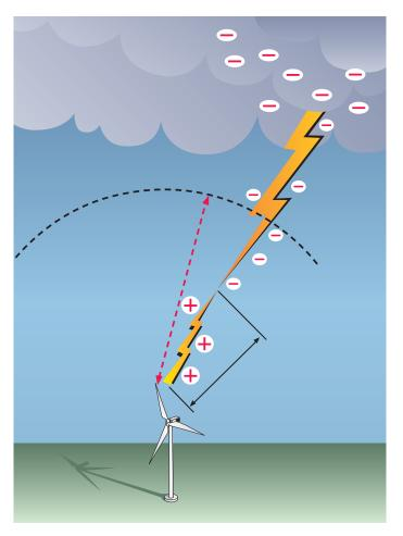
The dynamic phase of lightning commences in the form of a downward leader from the base of a cloud and grows into a series of steps and branches toward the ground. The protrusion of ground objects, such as wind turbine blades, into the ambient electric field of the lightning downward leader increases the electric field at the tip of the blade and/or other protruding parts of the turbine.
