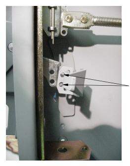
Install the bracket using these two holes and two 8-32 x .50 screws (Item 5) and star washers (Item 6) provided by Hoffman. Torque to 10 in-lbs.
