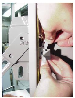
Note: The handle defeater arm is "sandwiched" between the dual defeater bracket and the nut plate.
