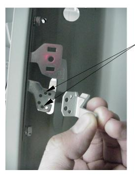
Install the bracket using these two threaded holes and the two screws provieded by Allen-Bradley. Torque to 10 in-lbs. Installed:
