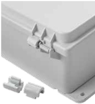
Hinge Retainers can be field-installed without modification to POLYPRO hinges for applications where cover removal is not desired. Two retainers per enclosure is recommended. Kit includes ten hinge retainers.
