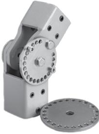
Accessory for use with Wall Joint, Cable Wall Joint and Intermediate Joint. Limits the rotation of these joints which normally rotate 180 degrees. Rotation Limiter provides stops in 15-degree increments. The limiter is a heavy-duty steel disk that attaches to the pivot point on each joint. Moveable stop pins provide adjustment.
