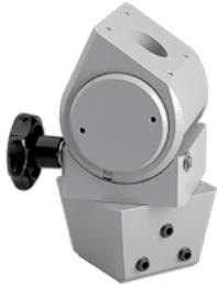
Mounts between suspension arm and HMI enclosure to provide both swivel and tilt options for machine operator. Cast aluminum assembly finished with RAL 7035 light-gray polyester powder paint. Center opening for control cables. Tilt knob allows infinite tilt adjustment from horizontal to 30 degrees. Swivel allows 300-degree maximum rotation. Setscrews, seals and enclosure mounting screws are included.
