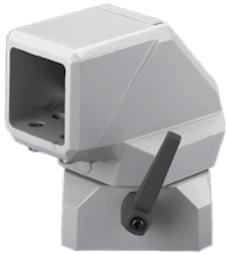
Coupling mounts to enclosure, enabling enclosure to be rotated 300 degrees. Enclosure can be locked in position. Removable access plates. Finish is RAL 7035 light-gray polyester powder paint. Setscrew, gasket and mounting hardware are included.
