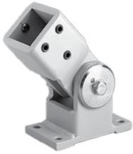
Welded steel plate construction finished with RAL 7035 light-gray polyester powder paint. Mounts equipment to vertical surface. Swivel range is approximately 180 degrees. Includes bellows with zipper, seals and setscrews. Adjustable tension at pivot point. Rotational limiter is optional. Mounting hardware not provided.
