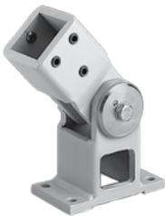
Welded steel plate construction finished with RAL 7035 light-gray polyester powder paint. Mounts equipment to vertical surface. Provides cable access to inside of pendant system from above or below. Swivel range approximately 180 degrees. Includes bellows with zipper, seal and setscrews. Adjustable tension at pivot point. Rotation limiter is optional. Mounting hardware not provided.
