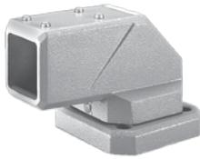
Cast iron finished with RAL 7035 light-gray polyester powder paint. Mounts equipment to horizontal surface. Permits pendant arm to be rotated or turned 306 degrees. Pivot bearing is maintenance-free. Setscrews, removable access plate and gasket are included. Mounting hardware is not provided.
