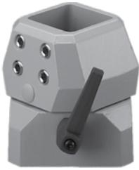
Flange Coupling mounts to enclosure, enabling enclosure to be rotated 300 degrees. Enclosure can be locked in position. Safety stop and maintenance-free bearing. Finish is RAL 7035 light-gray polyester powder paint. Includes installation instructions, setscrews, gaskets and mounting hardware.
