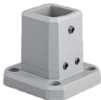
Wall Flange expands mounting options to include wall-mount as well as horizontal tube applications. Cast iron construction finished with RAL 7035 light-gray polyester powder paint. Setscrews, gasket and seals are included. Mounting hardware not provided.
