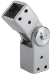
Welded steel plate construction finished with RAL 7035 light-gray polyester powder paint. Mounts to pendant tube. Swivel range is approximately 180 degrees. Setscrews and bellows with zipper are included. Rotational limiter is optional.
