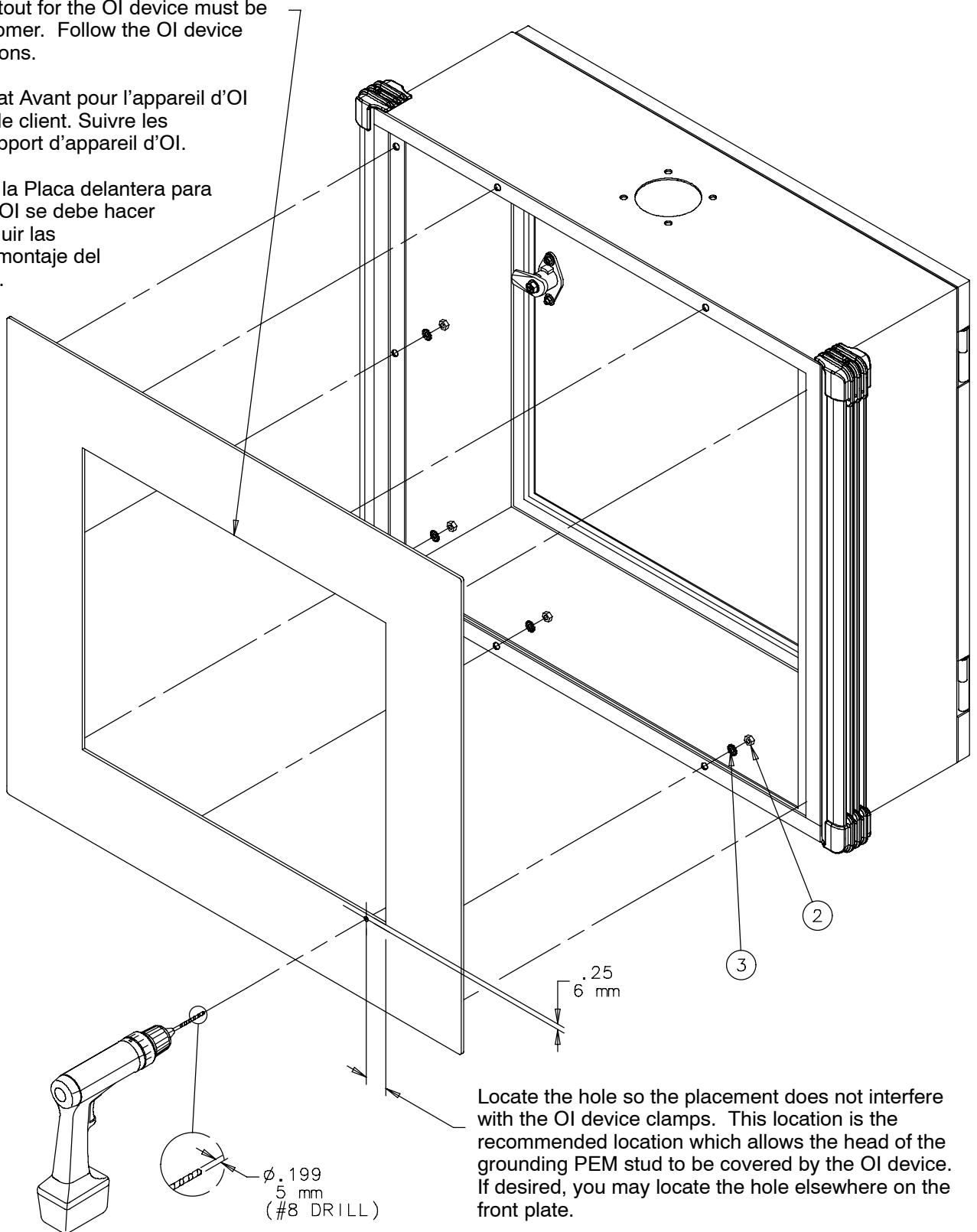
Locate the hole so the placement does not interfere with the OI device clamps. This location is the recommended location which allows the head of the grounding PEM stud to be covered by the OI device. If desired, you may locate the hole elsewhere on the front plate.
