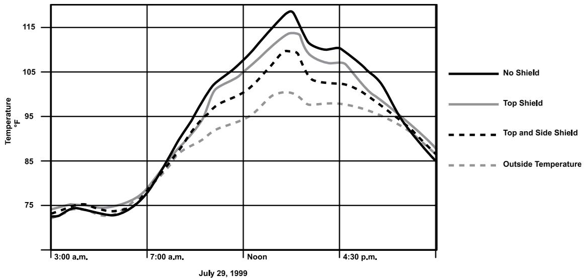
The results of the test show the enclosure with top and side shields to have approximately a 46% reduction in temperature compared to the unshielded enclosure. Hoffman offers top shields as an accessory for Hoffman COMLINE™ Wall-Mount Enclosures. The reduction in temperature is approximately 25% with the solar shield top only.
