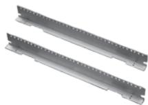
Rack Angles allow for mounting 19-in. rack equipment in 600-mm wide enclosures. Plated 14 gauge steel with .281-in. (7-mm) diameter holes (through-hole type). Twenty M5 screws and 20 clip nuts included for mounting rack angles to enclosure and for mounting equipment to rack angles.
