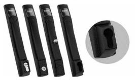
Flush Handles are optional for any solid, window or disconnect door that includes 3-point latching, except Voice/Data and Colocation cabinets. They are ergonomically designed to provide style and function in a low profile. The handle is die-cast zinc finished with RAL 9005 textured black polyester powder paint. Provision to add your logo is included. Handle can be installed to rotate either clockwise or counterclockwise.
