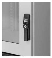
Swing Handles are used on smaller doors (doors 1000 mm and less in height that have two-point latching). Handles are ergonomically designed to provide style and function in a low profile. They can be installed to rotate either clockwise or counterclockwise. The shape of the design provides aesthetic compatibility with the Flush Swing Handles. This handle includes keylocking provision, two keys, provision to add your logo and is furnished in RAL 9005 textured black polyester powder paint.
