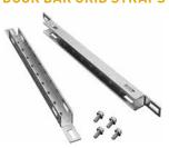
Straps mount to the door bar. Used to mount accessories to the door. Constructed of 16 gauge steel with plated finish. Holds up to 100 lb.
