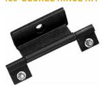
Optional hinging for steel solid, window or disconnect doors. The 180-degree hinges provide a door opening up to 260-degrees on single-bay enclosures. These hinges mount to the door flange and have a low-profile appearance. The kit includes three hinges with textured black polyester powder paint and all necessary mounting hardware. Cannot be used on PROLINE™ FLOTEK™ or CONNECTEK™ front doors.
