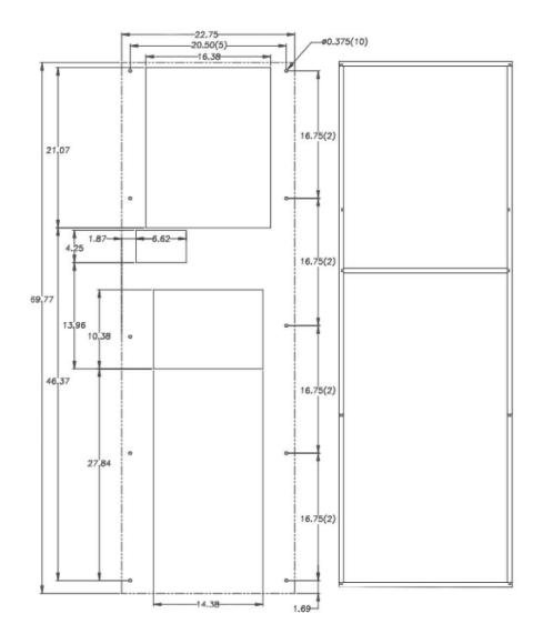
Mounting Gasket kit, 70-1000-50 included. Apply gasket to back of air conditioner before mounting to enclosure.
