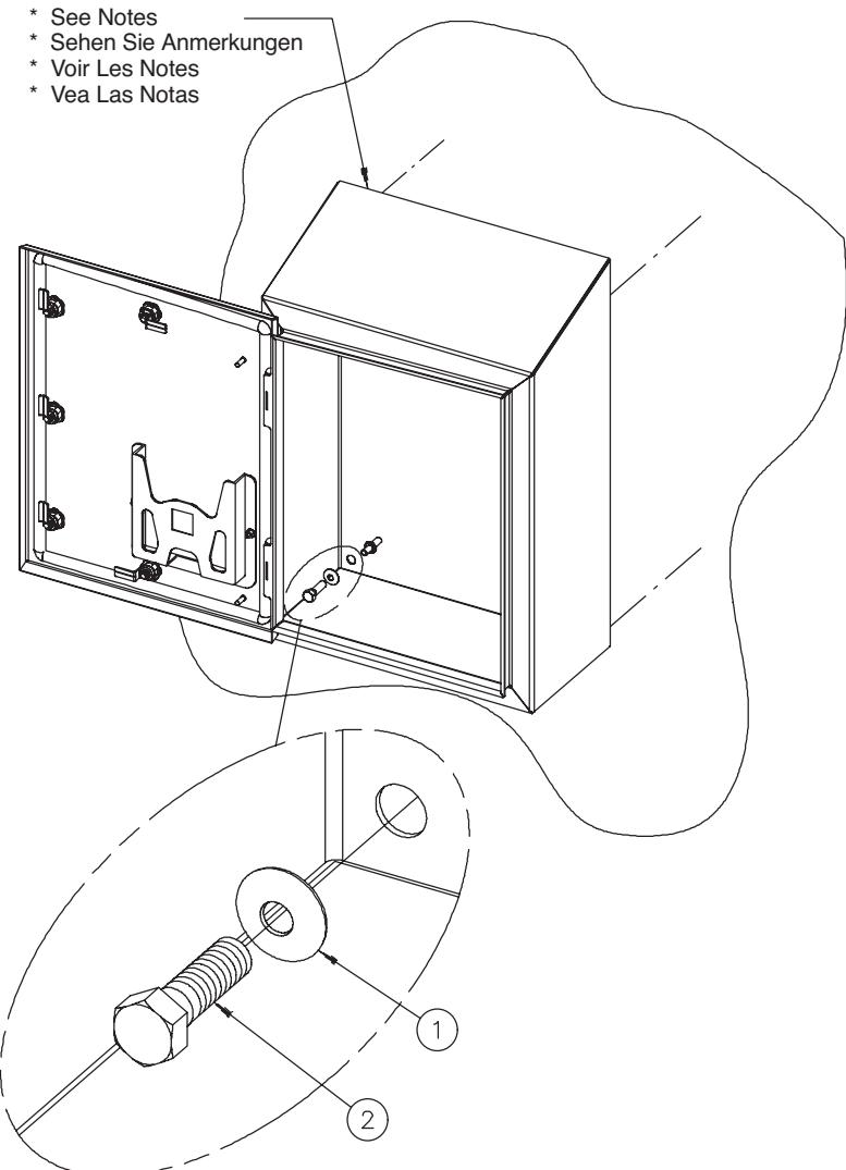
Mounting holes have been provided in the back of the enclosure for convenient mounting through the enclosure. Attach enclosure to wall or other structure using customer supplied 3/8 inch or M8 fastener, flat washers, and nuts. To insure proper sealing and enclosure protection rating, use the provided sealing washers. Install sealing washers inside the enclosure with rubber face against the enclosure.
