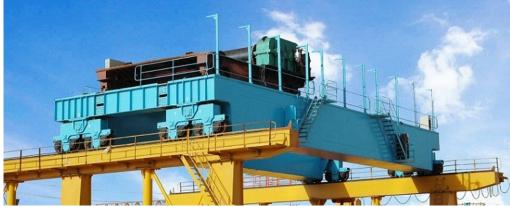
Double Girder Overhead Crane consisted with double girder bridge mechanism, traveling mechanism, trolley with frame and electrical parts. Compared to single girder overhead crane, its structure is stronger, more secure use, so double girder overhead crane lifting capacity is larger.
