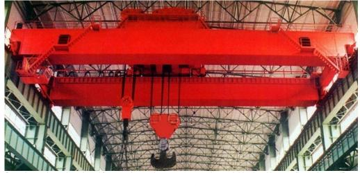
Operation mode can be selected for ground operations, remote operation, and driver's cabin according to the specific circumstances. Because of big span, large lifting capacity, high lifting height, usually more use driver's cabin operation. Each mechanism of crane operating speed can be designed into fixed speed; may also be designed to VVVF inverter type, using with hook **anti-sway**.
