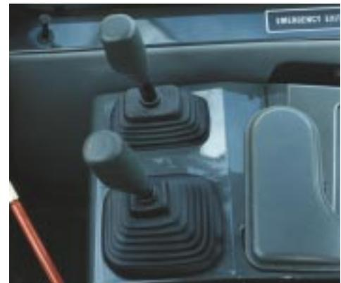
**Kick-down switch is conveniently located** on the mono-lever. A simple motion of the thumb actuates this valuable productivity feature.
