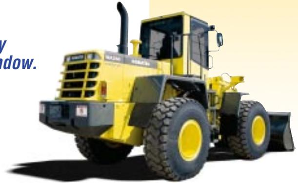
**plus** *Increased engine horsepower* Komatsu S6D102E-1 diesel power provides greater productivity and reliability. See page 6.
