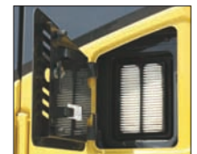
External air conditioner filter
