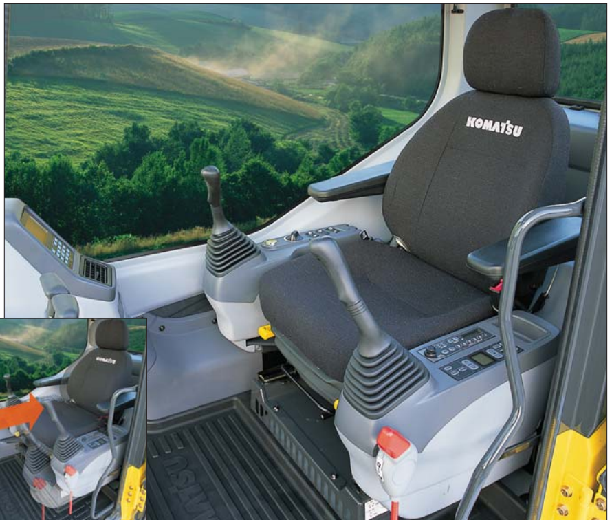
Seat Sliding Amount: 340 mm 13.4", increased 120 mm 4.7"
