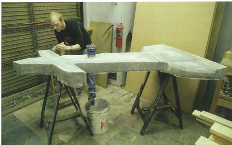
ABOVE LEFT: PROP ARTISAN ANTHONY CRAT PAINTING ONE OF CAROL 'S 10 GRAVESTONE WAGONS. THE WAGONS WERE CARVED FROM FOAM AND HAD CASTERS MOUNTED TO THEM, TO BE MOVED ONSTAGE BY THE ACTORS IN CAROL 'S "NIGHTMARE SEQUENCE." ABOVE RIGHT: SCENIC MECHANIC CHRIS FRYE CUTTING METAL TO CONSTRUCT THE LARGE (42 FT. WIDE) BRIDGE THAT WILL SPAN THE GEARY STAGE DURING CAROL 'S OPENING TOWN SEQUENCE. LOWER LEFT: DRAPER CUTTING THE FABRIC FOR MRS. FEZZIWIG'S SKIRT, WHICH WILL THEN BE AIRBRUSHED AND SPOT-DYED (WITH THE OTHER COSTUMES FROM THE "CHRISTMAS PAST" SCENES) TO APPEAR SATURATED WITH COLOR IN PLACES, AND MORE DIFFUSED IN OTHERS. "BEAVER BAUER'S DESIGNS FOR THESE SCENES EMPHASIZE THE DEGREE TO WHICH, IN SCROOGE'S MEMORY, NOT EVERYTHING IS REALIZED, SO COLOR ONLY COMES THROUGH VIBRANTLY IN PARTS," SAYS DRAPER. LOWER RIGHT: AN OVERHEAD VIEW OF THE A.C.T. PAINT SHOP. SCENIC ARTISTS JENNIFER BENNES AND B. J. FREDERICKSON ARE PAINTING THE TOWN SLIDERS THAT WILL EVOKE "A DREAMLIKE, IMPRESSIONISTIC, AND ALSO SOMEWHAT FRIGHTENING REPRESENTATION OF SCROOGE'S LONDON," SAYS SCENIC DESIGNER JOHN ARNONE.
