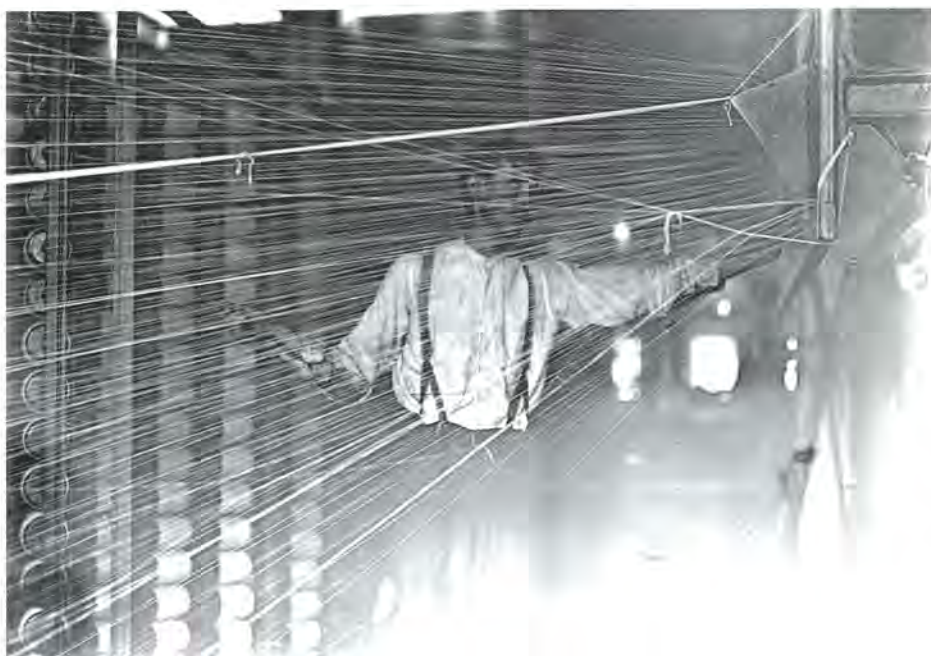
A WORKER STANDS BEHIND THREADS BEING FED INTO THE WARP SIDE OF A MACHINE LOOM AT A COTTON MILL, 1908. PHOTO BY LEWIS WICKES HINE (© CORBIS).
