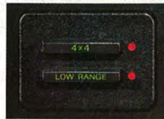
Touch Drive lets you shift from 2WD to 4WD High, and back, with pushbutton ease.
