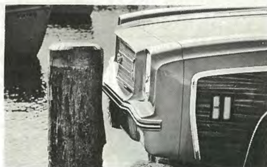
Grille and lights are housed in a nose cone of resilient urethane
