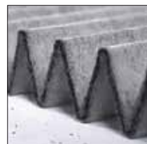
MERV 13 layer bonded to 200 g/m 2 carbon matrix with support scrim
