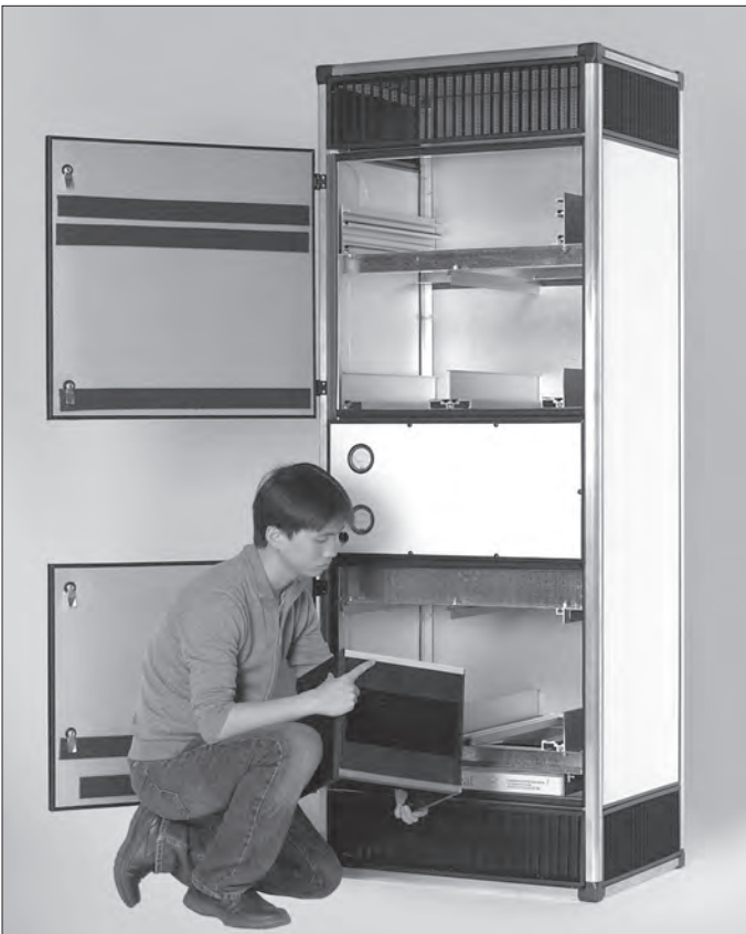
Step 1: Bring the HD half-cassette to the RU and prepare to install it. Turn the half-cassette so that the yellow butterfly gasket will be on the bottom and pointing into the enclosure.
