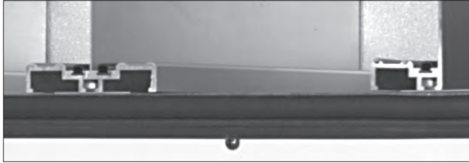
Track connection detail at support beam. This detail shows AAF's "quick release" track installation method. Accurately located support post holes ensure high tolerance track spacing. Note that the track connection is completely isolated from the filter sealing surface and cannot interfere with filter installation.
