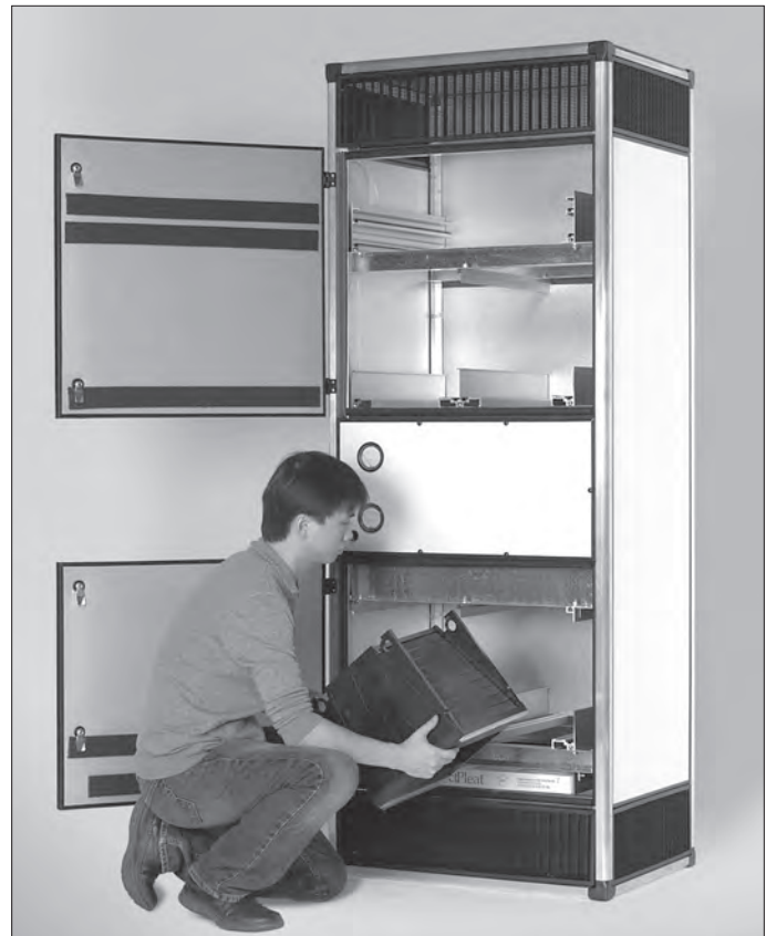
Step 1: Bring the HD half-cassette to the RU and prepare to install it. Turn the half-cassette so that the yellow butterfly gasket will be on the bottom and pointing into the enclosure.
