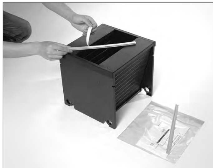
Step 1: Remove the paper strip on the back of the yellow "butterfly-style" face gasket to expose the adhesive.
