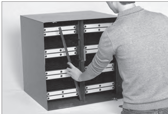
Step 1: Take one cassette sealing and locking channel.
