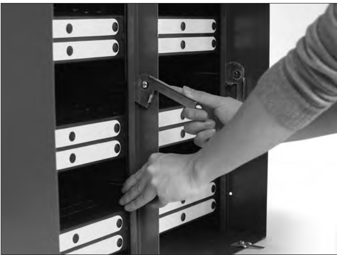
Step 5: Making sure that the locking handle is hooked behind the front flange of the locking handle support tab and cannot slip off, rotate the locking handle downwards so that the face of the handle engages the web of the channel, forcing it against the cassettes and pushing them into the housing to compress the face gasket.
