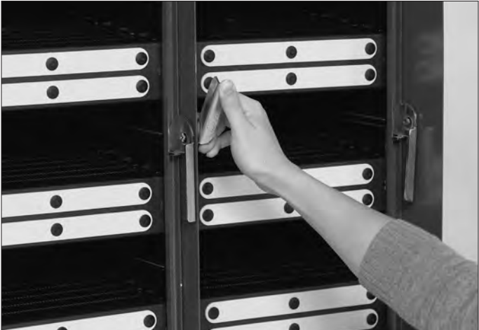
Step 7: Now, repeat the process on the right hand side of the center vertical cassette support panel. The handle on the right hand side of the panel rotates upwards.
