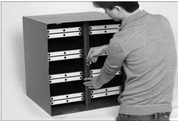
Step 4: Insert the filter seal locking handle into the locking channel so that the locking handle support tab protrudes completely through the hole in the locking handle.
