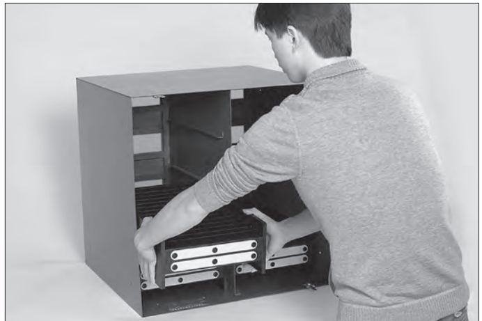
Step 2: Slide the filter into the FAH.
