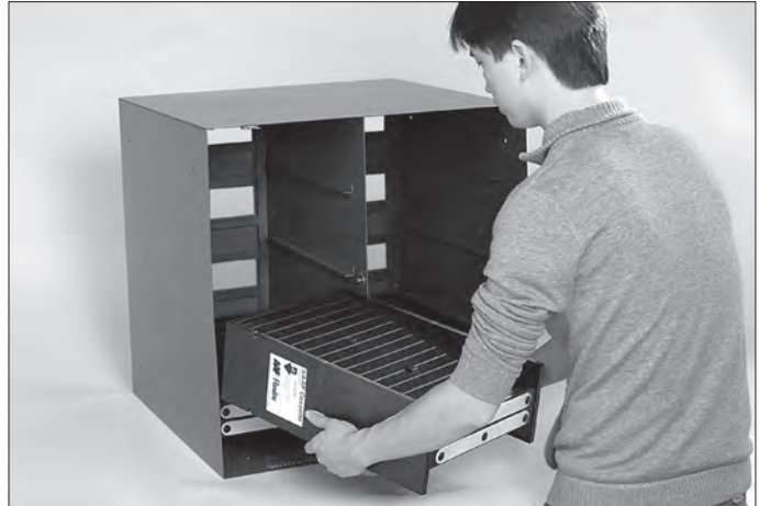
Step 1: Insert the filter into the FAH.
