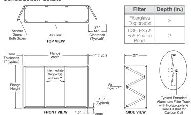
\*Allow 27" minimum clearance on one or preferably both sides for filter installations.
