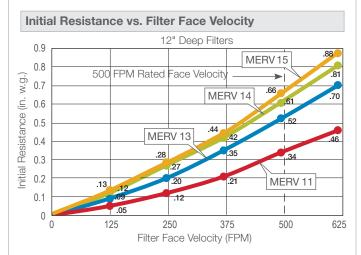
12" deep filters are rated at 500 FPM filter face velocity.
