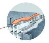
Media Pack Sealant - A layer of high efficiency media seals the media pack into the cell sides. The media sealant prevents by-pass leakage and damage to the media and separators during shipping and handling. By allowing slight movement of the media pack when the filter is jarred, the cushioning sealant helps prevent tears and punctures to the media.
