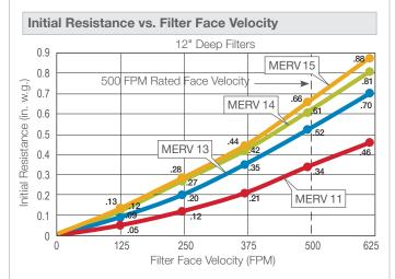
12" deep filters are rated at 500 FPM filter face velocity. 6" deep filters are rated at 250 FPM filter face velocity. Recommended final resistance for VariCel filters is 1.5" w.g. Recommended final resistance for HT VariCel filters is 1.2" w.g.
