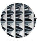
Corrugated Aluminum Separators with Rolled Edges maintain uniform pleat spacing for optimum airflow. The separators are rolled to eliminate sharp edges, preventing media damage during shipping and personal injury during installation.
