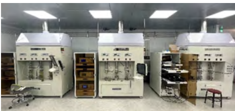
Accelerated media life test station and gas monitoring equipment
