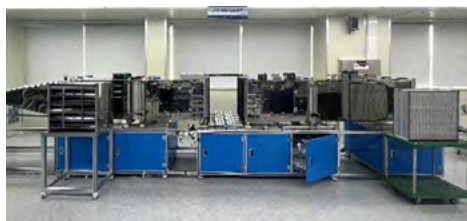
Full-scale filter test rig for pressure drop, removal efficiency, outgassing, and particle emission measurements
