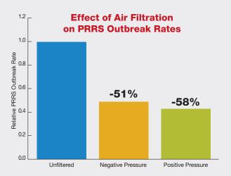
Negative Pressure Filtration: Maintains lower air pressure inside a facility compared to outside, ensuring that all incoming air is pulled through filters to prevent the entry of airborne contaminants.
