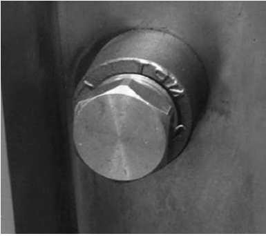
Static Pressure Taps are 1/4-inch Stainless Steel Half-Coupling with Brass Hex Plugs
