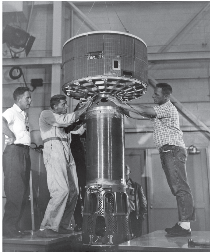
Assembly of the Television Infrared Observation Satellite (TIROS) in a clean environment, April 1960
