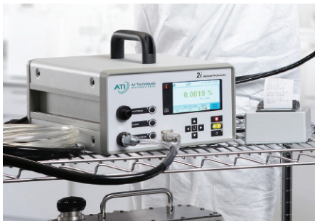
ATI's 2i Photometer Detects Leaks in HEPA Filters
