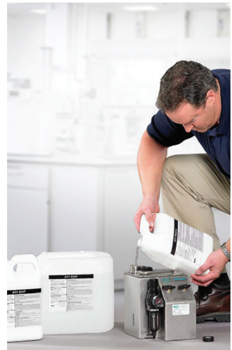
Filling a Laskin Nozzle Generator with an Oil Reagent to Create a Challenge Aerosol
