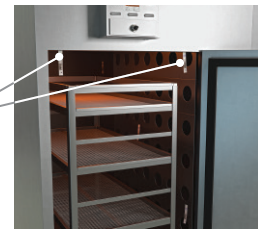
Biological indicators can be placed in multiple areas of the chosen equipment or filter medium
