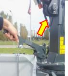
Attention! crushing of the hands and collision of the head with the boom with winch above during its rotation.
