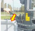
Once in horizontal position, use the release lever to move the boom with winch in the required direction and let go of the lever at the point closest to the one required.
