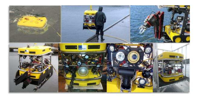
All Ocean Modules ROV systems have opened steel frames that makes them less affected from ocean currents. Together with the continuously compensating control system, that regulates the thrusters to always maintain the ROV in position, this makes Ocean Modules ROV systems best-in-class. The V8 L3000 has proved suitable for several tasks traditionally carried out of by larger Work-class ROV systems and Ocean Modules will continue to push the boundary of what is possible and to get the job done.
