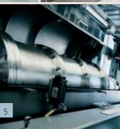
1/ In the separation module the sludge is separated into clean oil, solids and water.
