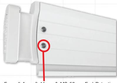
The Eyewall Armor® 44mm & MS 56mm End Retention System are two of the only systems available that employ Aluminum Rivets to secure the End Retention guides to the slat. This avoids the issue of inserting Stainless Steel screws into the end of the slats, which causes severe corrosion through the contact of dissimilar and incompatible metals.
