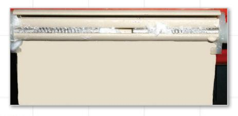
This picture shows the dramatic effect of exposing dissimilar metals to a salt environment. This corrosion adversely affects the ability of a screw in an end retention guide to perform over extended exposure in coastal environments.
