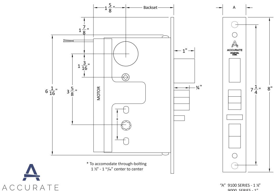
M9167E- Motor Drive Electrified Mortise Lock With Mechanical Deadbolt
