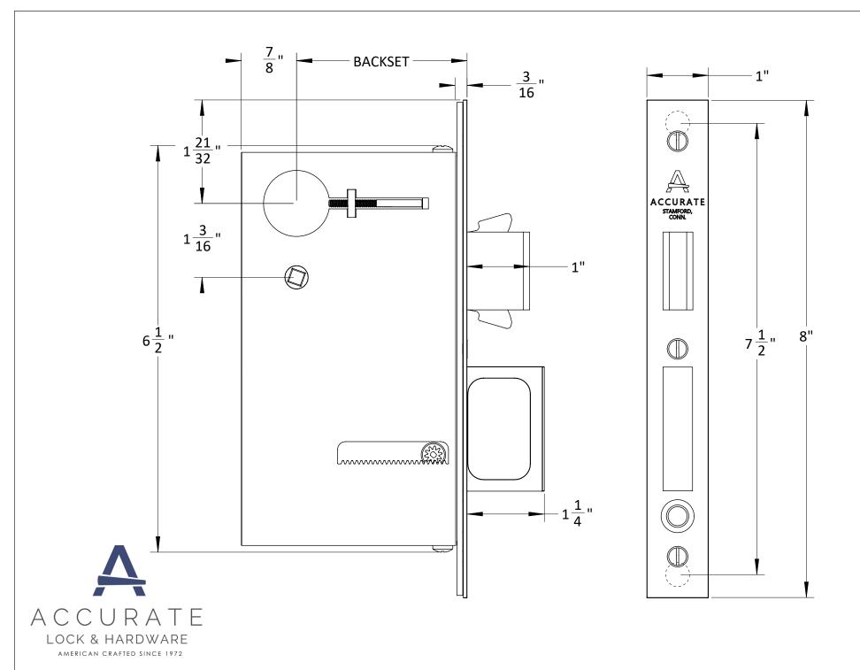
2002Q Quiet Pocket Door Lock With Integrated Edge Pull
