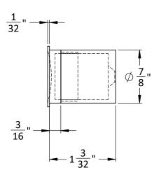
The part is provided with the full magnet strength but is adjustable down for lighter doors. The magnets are removed prior to installation.
