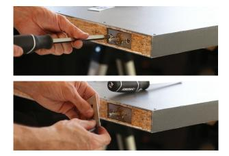
**3. Tighten Armor Front Screws** Tighten the base front scews and then attach the faceplate.
