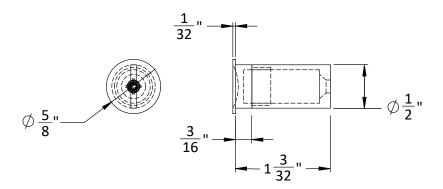
The part is provided with the full magnet strength but is adjustable down for lighter doors. The magnets are removed prior to installation.
