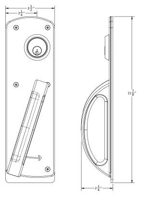
Offering advanced safety features like paperclip protection, the Narrow Crescent Mortise Set can be used on Thermal narrow stile doors (installed 4-1/4" from edge of the door).
