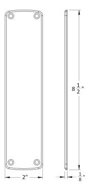
Lightweight, solid brass construction designed with institutional strength and durability.
