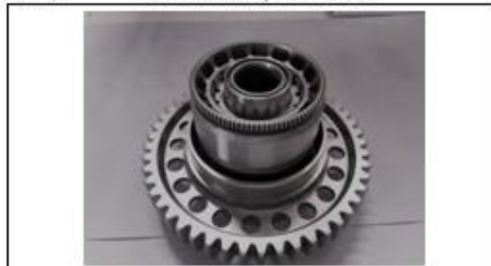
W1-5) Differential assembly on crown wheel
