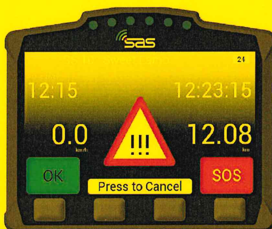
SCREEN 15. Manual Hazard in Transport Mode
